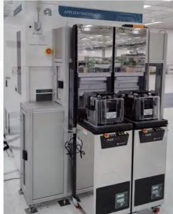
AMAT Verity 2x PLUS 500S with Mini-Environment
