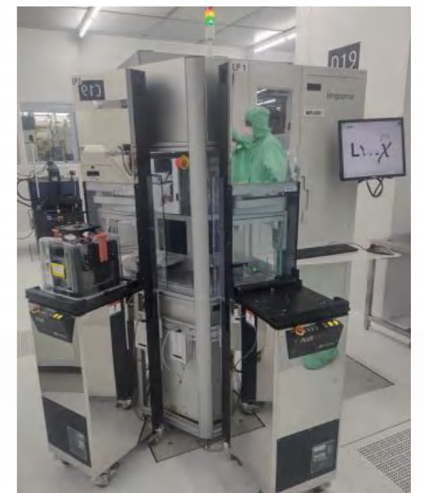
ONTO Imperia 2x PLUS 500S + Mini-Environment
