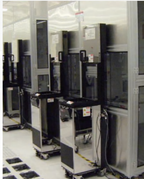
Novellus-CONCEPT 2 2x PLUS 500S and Mini-Environment
